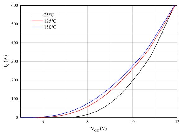
图 3. 典型传输特性 ( $V_{CE}=20V$ )Figure 3. Typical transfer characteristic( $V_{CE}=20V$ )
